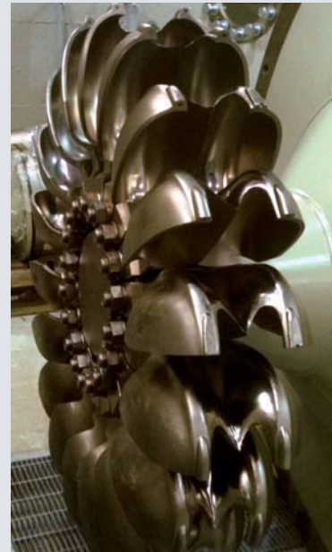
Fabbriche I - Pelton turbine ready for installation
